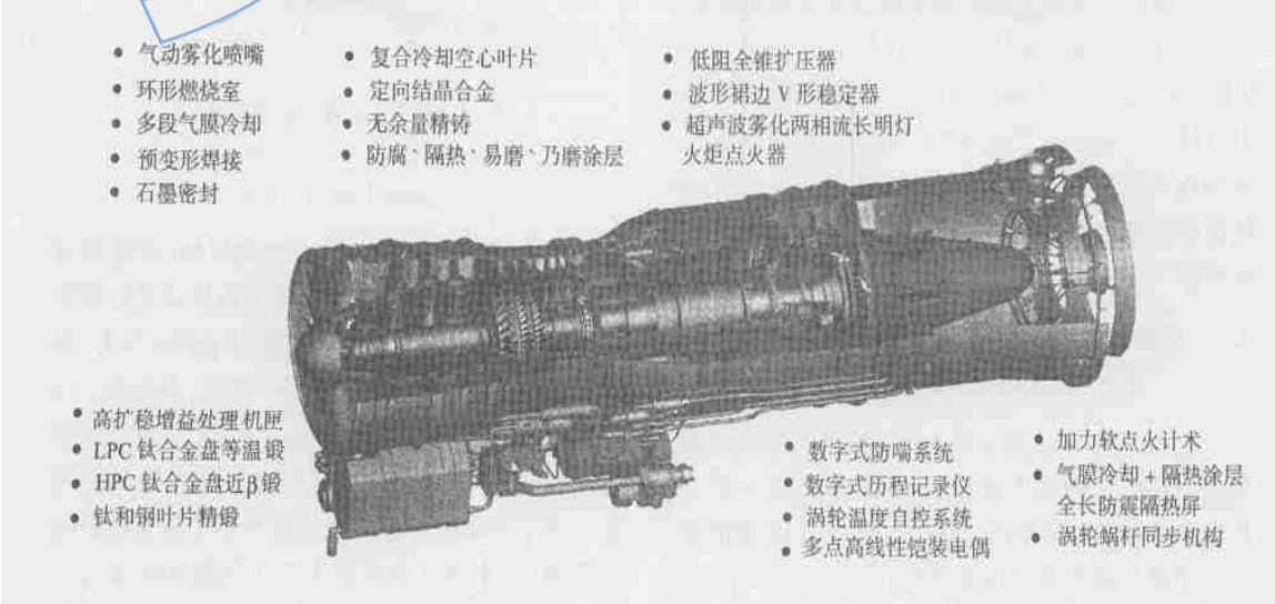
图3 昆仑发动机的剖视立体图及新技术 Fig 3 The cutaway view and advanced technique for Kunlun engine
