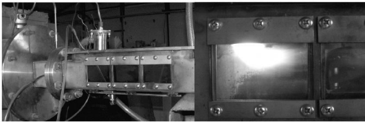
图 2 直段空腔试验段及扩散射流火焰 Fig. 2 Schematic diagram of the straight passage and the diffusion jet flame
