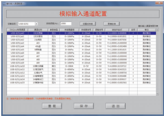
图 7 测量通道配置模块 Fig. 7 Module of the measurement channels configuration
