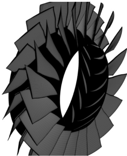
图 1 对转压气机的全通道两级转子叶排网格 Fig.1 Rotor 1 and rotor 2 of the counter-rotating compressor
