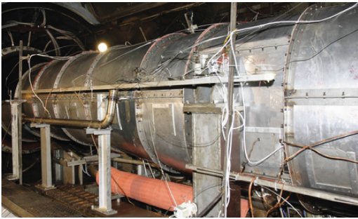
图 2 带发动机保温罩台架安装图 Fig. 2 Installation of turbfan engine with insulated box
