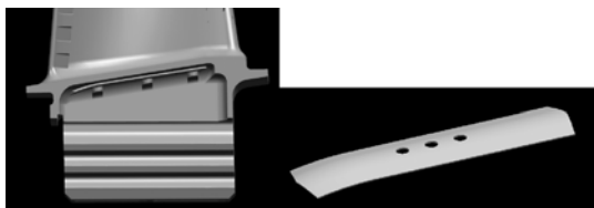
图1 某高压涡轮工作叶片缘板阻尼结构 Fig.1 Structure of platform damper for a high pressure turbine blade
