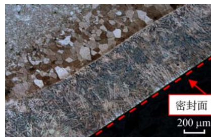
图1 全新排气门密封面区域的金相组织 Fig. 1 Metallography of sealing area of a new exhaust valve
