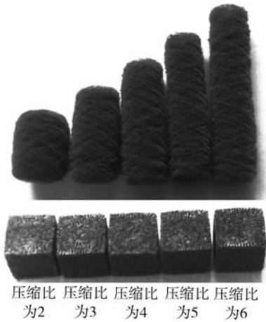
图 1 金属橡胶试件与对应毛坯 Fig. 1 Metal rubber samples and its roughcast
