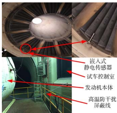
图7 静电传感器机载化安装实物图 Fig. 7 Photo of airborne installing for electrostatic sensor
