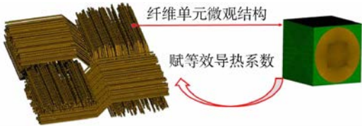
图 11 纤维单元赋等效导热系数 Fig. 11 Assign effective thermal conductivity to the fiber element
