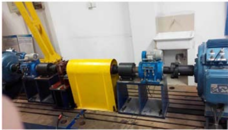
图 5 电封闭齿轮综合性能试验台架 Fig. 5 Test bench for the comprehensive performance of electric closed gears
