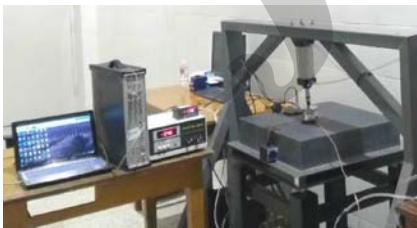
图 4 气膜微振动测试装置 Fig. 4 Experimental rig for micro-vibration of gas film
