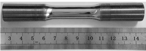
图 1 DD6 薄壁圆管试样 Fig. 1 DD6 thin-walled tube specimen
