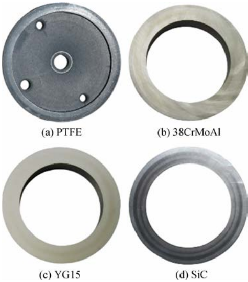
图 7 PTFE 与硬材料摩擦后的表面形貌 Fig. 7 Surface morphology after the friction between PTFE and hard materials
