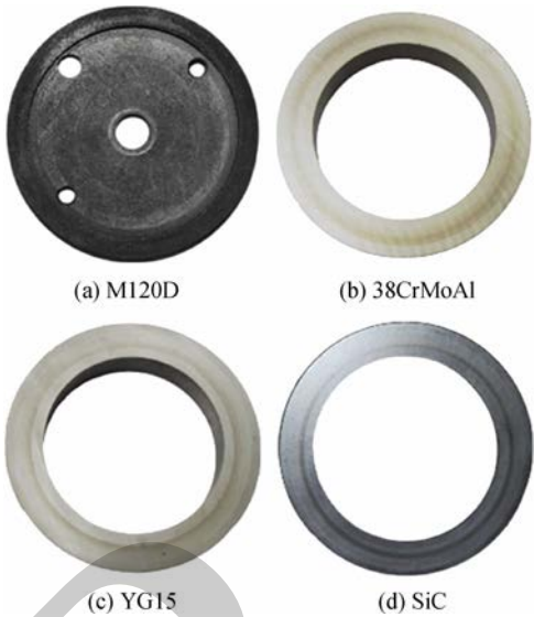
图 6 M120D 与硬材料摩擦后的表面形貌 Fig. 6 Surface morphology after the friction between M120D and hard materials
