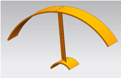
图 7 带前缘特征平板模拟叶片转子三维示意图 Fig. 7 Three-dimensional schematic of blade rotor with leading edge characteristic plate simulation
