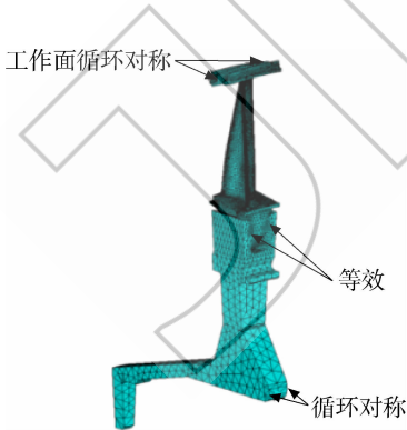
图 6 传统模态分析叶片盘边界条件 Fig. 6 Blisk boundary conditions for traditional modal analysis
