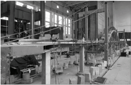
图6 桃花峪黄河大桥全桥模型试验示意 Fig.6 Model test of Taohuayu Yellow River Bridge
