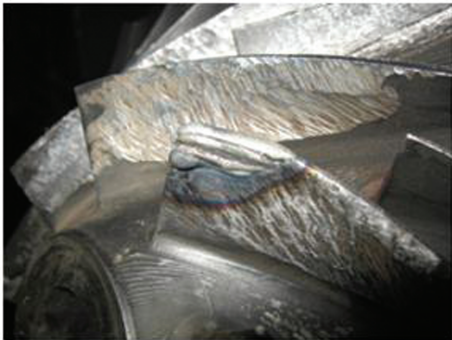
(a) 叶片(1)成形后整体形貌
