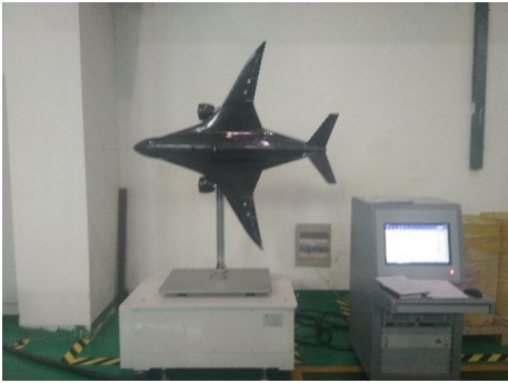
图 4 某翼身融合布局模型转动惯量测量 Fig. 4 Measurement of moment inertia of blended wing body model
