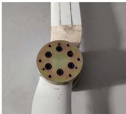
图2 反演桨转接盘局部照 Fig. 2 Photo of adapter for inversion propeller
