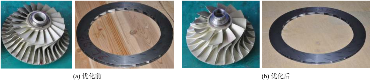
图 19 单状态优化前后离心叶轮和径向扩压器实物 Fig. 19 Machined centrifugal impeller and radial diffuser before and after the single-state optimization
