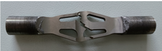
图 10 盘心多轴应力模拟件试验结果 Fig. 10 Test results of disk centered multiaxial stress simulator
